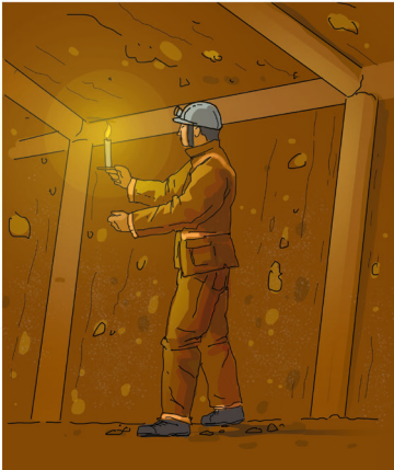
Picture 27: Candles can be used to determine the level of oxygen in the air
