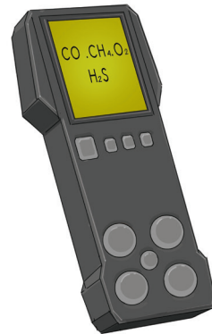
Picture 26: Special measuring equipment gauges the level of different gases
