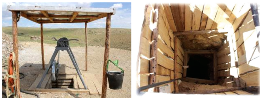
Picture 24: An improved ASM shaft
