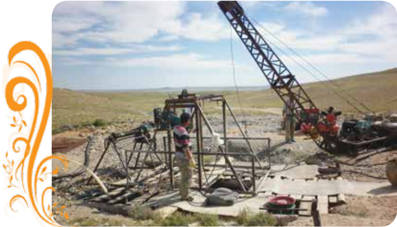
Photo 40: A mechanised hoist that is designed to carrying ore from the shaft
