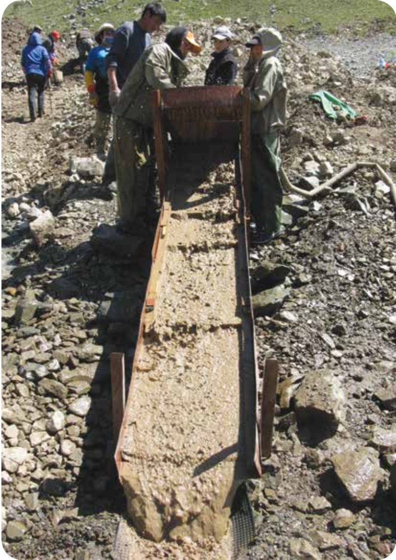
Photo 11: The testing of sluices
