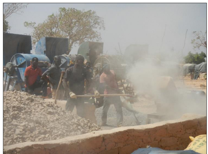
Figure 12: Dust exposure in artisanal hard rock mining is a common threat (Photo: AGC)
