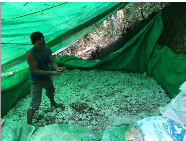
Figure 11: A miner stands on a batch of ore in a heap leaching pit, which uses cyanide as leaching agent (Photo: AGC)
