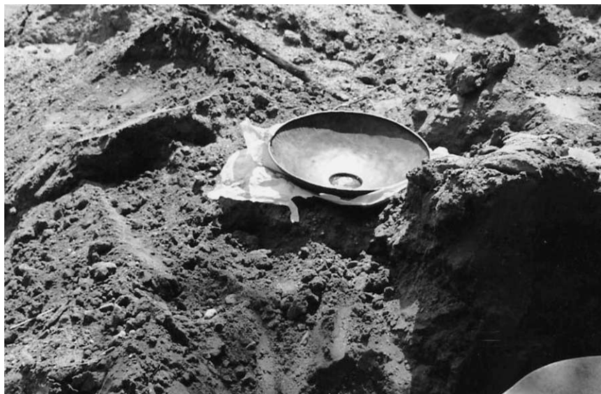
Fig. 4. Appropriate processing technology—metallic gold panning dish.
