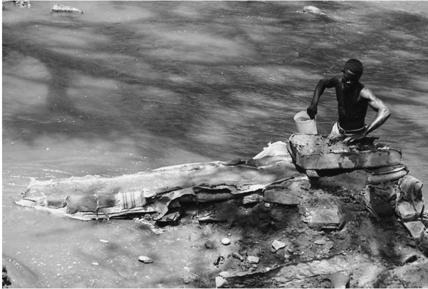
Fig. 5. A portable James Table in use on Angwa River, Zimbabwe.
