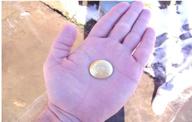
**Figure 7:** The gold rich concentrate will be melted with a gas smelter to a gold bar. In this case to a bar of about 45 grams with a worth of 2.1 million MNT.
