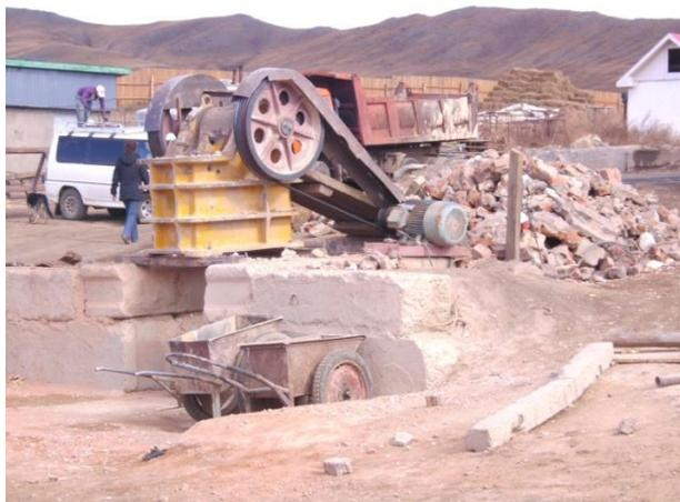
**Figure 5:** The jaw crusher of XAMO Company. Underneath there are two typical wheelbarrows.
