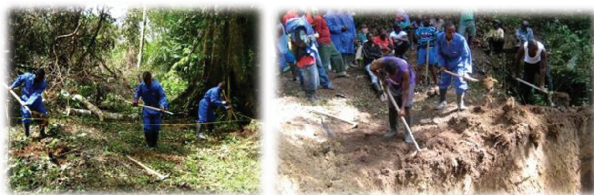
Figures 10 and 11: Miners in Liberia demarcating trenches and backfilling as they mine 22
